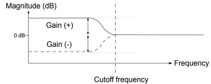
Two parameters are available, the frequency of operation and the gain. Gain specifies how much to attenuate or boost the chosen frequency. At center position (0 dB) the signal is not affected in any way.
