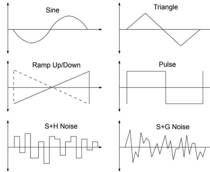
Figure 4.10: LFO waveforms.
