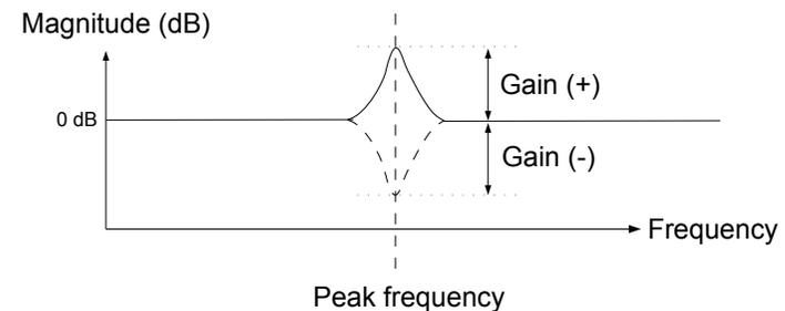
The peaking EQ offers a frequency and gain parameter like the Low Shelf EQ, additionally a
