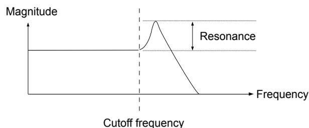
Figure 4.6: Response of a resonant low-pass filter.
