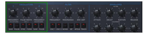
Obsession uses two oscillators as the core of its synthesis, which produce periodic pitched tones. The sound parameters are explained below.
