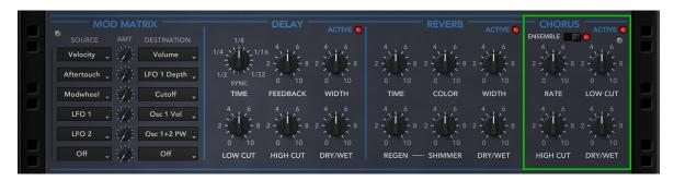
A chorus effect is obtained by summing a signal with a delayed copy of itself. When the delay is continuously varied with a low-frequency oscillator and separately for the left and right channel, the sound becomes thicker and more spatial.
