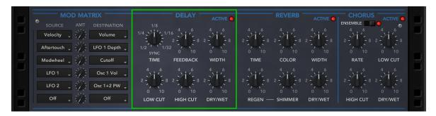
The Stereo Delay in Obsession creates a series of echoes, synchronized to the host tempo.
